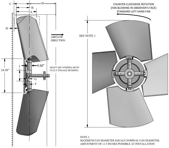
BUSHING AND/OR AIR SEAL CAN BE INSTALLED ON INLET OR OUTLET SIDE OF FAN
